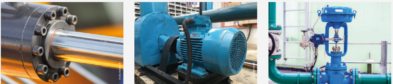
Fig. 12: Typical actuators (hydraulics, fan, valve)
