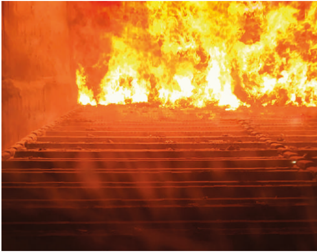
Fig. 7: Principle grate combustion system
